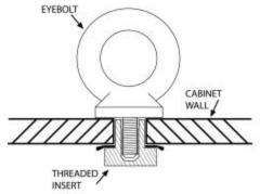
mm x 1mm pitch x 12 mm thread length steel forged shoulder eyebolts
